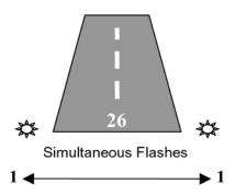
If the aircraft is off the runway centreline by more than 0.45°, up to a maximum of 15°, the pilot will see a delay between the flashes. The two lights will flash with a variable delay (60 to 330 ms) according to the position of the aircraft relative to the centreline. The further the aircraft is from the centreline, the greater the delay. The delay between the two flashes produces a sequence effect, which shows the direction towards the runway centreline.
